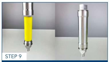
Set the discharge end with stator and rotor assembly on the table and slide the body assembly over it. Tighten 160 in/lbs (13ft/lbs). Be sure to leave it vertical (discharge end pointed down) until tightening otherwise the nozzle could misalign.
