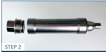
Remove the inlet cap. Put in a vise with flat spots on nozzle body contacting jaw face. If you do not have a vice, you may use a pipe wrench on the nozzle body to hold it. Use a 1-1/8" wrench to loosen and remove the inlet end cap.
