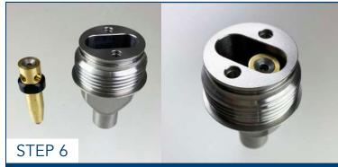
Install the rocker assembly into the nozzle end cap assembly with flat sides lining up with guide pinholes.
