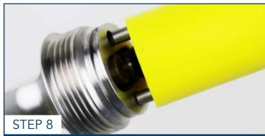
Hold the discharge end with the rocker assembly at a 45-degree angle with guide pins horizontal. Align guide pin holes with guide pins on stator while ensuring rotor tip aligns with rocker assembly.
