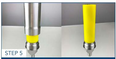
Once discharge end cap is fully loosened, remove from vise keeping the discharge end cap down and lift nozzle body off discharge end cap. The internal nozzles and stator will remain attached to the discharge end cap and the whole assembly will be replaced.
