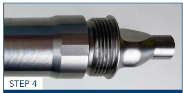
Remove discharge end cap assembly. Put in a vise with flat spots on a nozzle body contacting jaw face. If you do not have a vise, you may use a pipe wrench on the nozzle body to hold it. Use 11/16" wrench to loosen discharge end cap.
