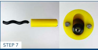
Install the new rotor into stator with the metal seat of the rotor pointing to the side with the guide pins.
