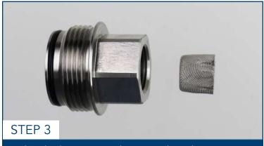
Replace the dome screen and o-ring on inlet end cap. You may use a wire brush to clean the threads of the end cap and inside the nozzle body (if needed). Reinstall inlet cap onto nozzle body, using a 1-1/8" socket or wrench, tighten to 160 in/lbs (13 ft/lbs).
