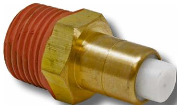
Protects the pump from damaging heat build-up while it is in bypass mode. The thermal relief valve, sensing a rise in temperature, opens and discharges a small amount of heated fluid. This allows cooler water to enter the system and cool the pump. When the gun is discharged the cooler water will cause the valve to close immediately.
