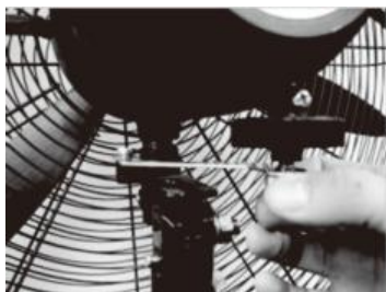
FIG 3 – For an OSCILLATING fan head, turn the OSCILLATING ADJUSTMENT screw anticlockwise to attach SWING ARM to fan head
