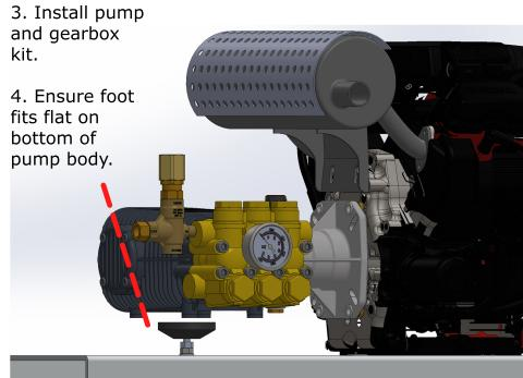
5. Adjust nut so foot and pump body gently contact.
