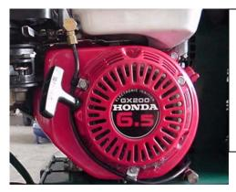
Secure the throttle control in two places around the recoil as shown in the picture. This keeps the airline out of harms way and provides extra support to the throttle control.
