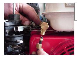
Run the airline from the unloader valve up to the throttle control.
