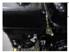
Place the filter and cover back on the engine.
