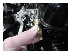
The nut which holds the bracket onto the throttle control body should be loose enough to allow the fitting to be angled in the appropriate direction. Aim the fitting in the desired direction and tighten the nut to secure it in place.
