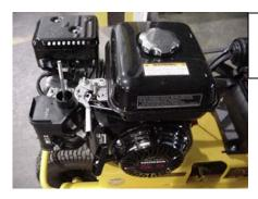
Remove the cover and air filter from the engine to allow easy access to the throttle arm.
