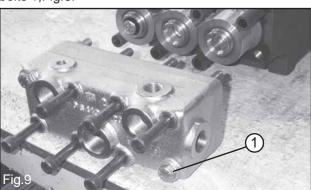
Replace them with two screws with nut (1, Fig.9) to keep head and collector packed up together and then remove the other six head bolts. Now head and collector can be easily separated from the pump and then disassembled on the working desk (Fig.10).
