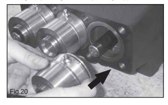
Once reassembled fit the pumping units back in the pump (Fig.20), tighten the plunger screws at 5 Kgm and finally the head bolts at 9 Kgm by mean of a torque wrench. Grease the packings as per instructions of par.11.3.
