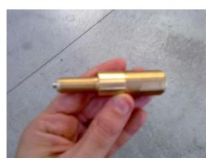
3 The nozzle can be further disassembled from the assembly by means of a no. 2 Allen wrench.
