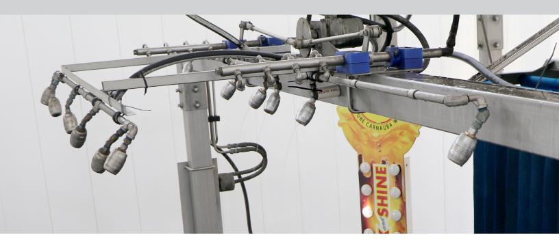
The Blast-Tec Pro was designed specifically for high-pressure, high-impact vehicle wash applications including wheel blasters, undercarriage wash, rinsing, and high-pressure cleaning.
