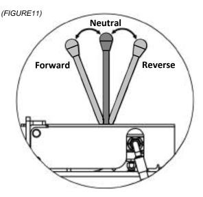
**FORWARD** — Move the control handle to the FORWARD position which will engage the wedge forward to split the log.
