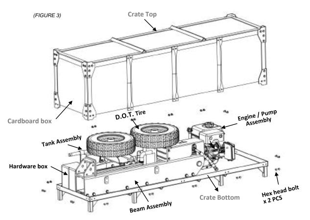
Step 2: Carefully remove all loose parts included in the container, e.g. hardware box.
