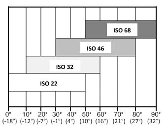
Approved fluids include Shell Tellus® S2 M 32 Hydraulic Fluid, Dexron® III / Mercon® automatic transmission fluid, Pro-Select<sup>™</sup> AW-32 Hydraulic Oil or 10WAW-ISO viscosity grade 32 hydraulic oil. It is not recommended that fluids be mixed, to top off the reservoir tank during initial set-up use Shell Tellus® S2 M 32 Hydraulic Fluid only.
