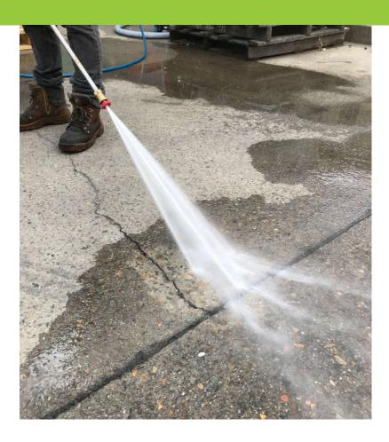
**ABOUT** - New from BAR, the patented "multi hole" nozzle is designed to cut out troublesome gum and other grime without the normal problem of cutting into the cleaning surface
