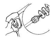
Open the water gun pressing the gun trigger and keep it in this position for some seconds in order to eliminate the air in the hoses.
