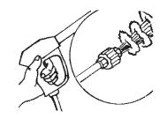
At the end of the work, cut-of the hydrocleaner turning the switch in the "OFF" position than, open the water gun to discharge the residual pressure in the H.P. hose.
