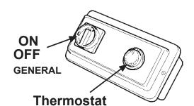
Set the start switch to ON keeping the thermostat to a minimum.
