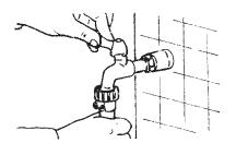
Connect the other extremity of the supply hose to the water tap. Make sure that the quantity of water which feeds to the hydrocleaner is equal to the pump capacity.
